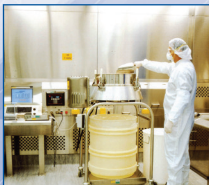
Weighing and Sieving Operations inside a Downflow Booth
