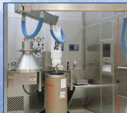
Dispensing Booth with Integrated Vacuum Lifter and Post Hoist
